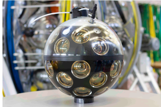
Fig. 24. The KM3NeT optical module (from Ref. 271 ). The optical module consists of a glass sphere with a diameter of 42 cm, housing 31 photosensors (yellowish disks). The glass sphere can withstand the pressure of the water and is transparent to the faint light that must be detected to see neutrinos.
